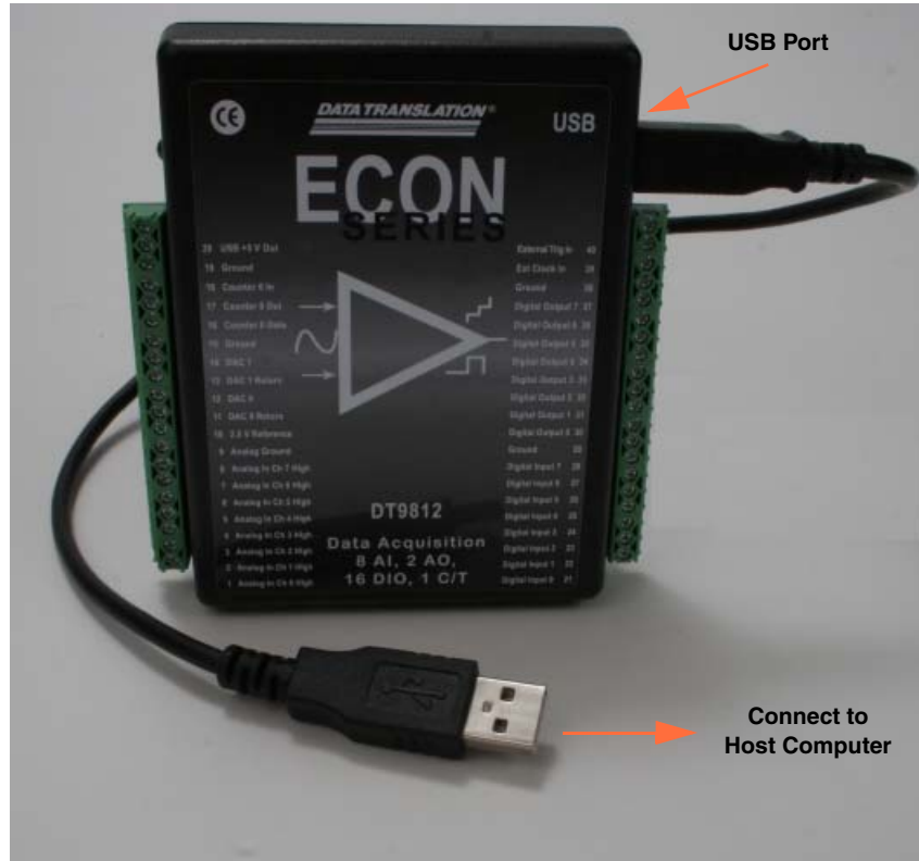
Figure 3: Attaching the Module to the Host Computer
