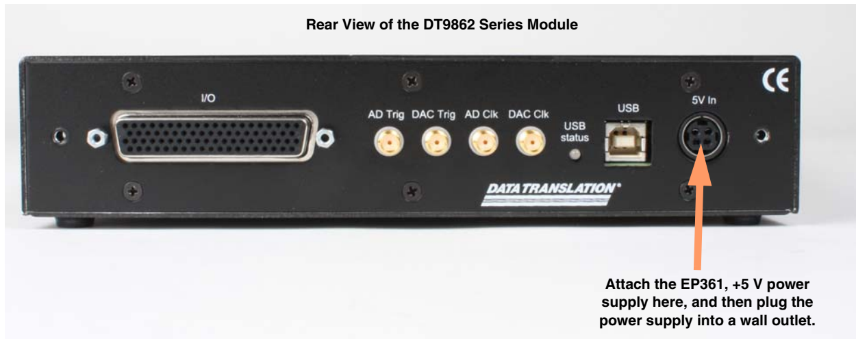
Figure 3: Attaching a +5 V Power Supply to the DT9862 Series Module
